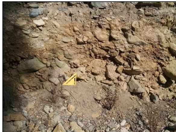
Figure 15. Typical right bank sediments in the reach between Temescal Canyon Rd and I-15. Note the predominantly larger material within a coarse sand matrix.
